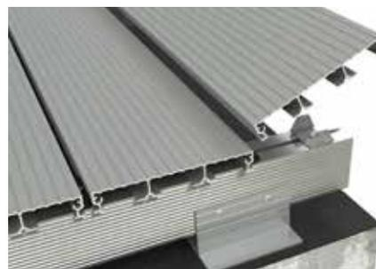
Slot the edge of the under the last clip and press the board down over the snap-on clip to fix in place. Tighten the screw on the clip between the last two boards to clamp firmly in position.
