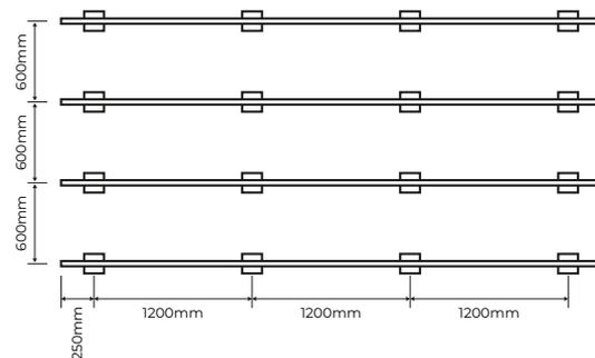
2. Set out a cleat foot at each point required using appropriate spacings along the length of the **BoxRail™**, using the table below.
